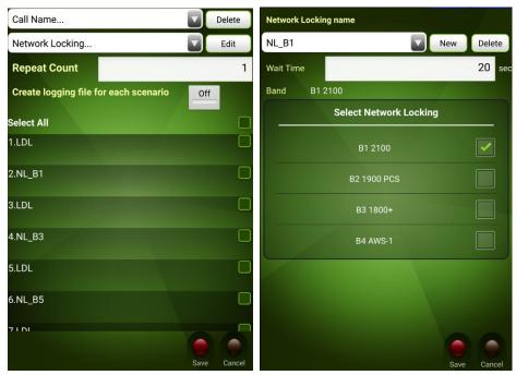
While processing Multi-Call test, [Network Locking] shows the status of Band Lock.
